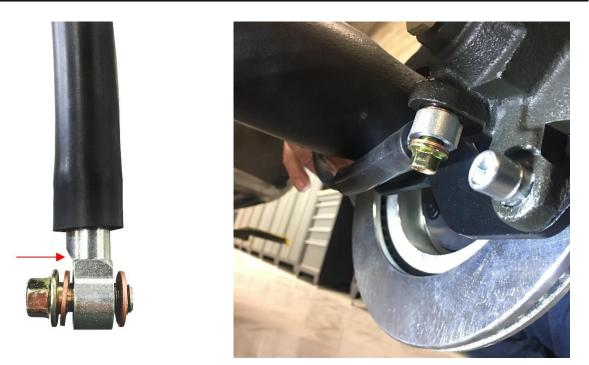
Install the banjo bolt and crush washers onto the hose as shown. If your hose has an offset, place the offset side of the fitting **away** from the caliper. Then install the hose onto the caliper as shown.
