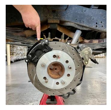
An easy way to accomplish this is to unbolt the main caliper bracket from the axle (leaving the caliper bolted to it) and rotate the caliper around the rotor until the bleeder screw is vertical, then perform the bleeding procedure. Keep the caliper with pads on the rotor during bleeding so that the piston doesn't over-extend outside of its bore.
