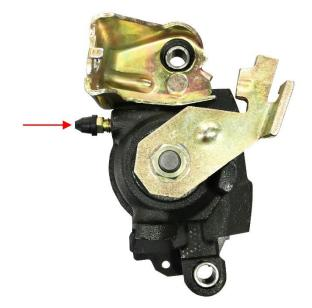
When bleeding this type of parking brake caliper where the bleeder screw is horizontal once installed, we have found that they bleed best when the bleeder screws are **parallel to the ground**. If it is not, then it will be necessary to reposition the vehicle, the axle, or the caliper. **If the bleeder screw is not parallel to the ground while bleeding, then you can bleed gallons of fluid through it without eliminating all of the air.**
