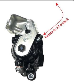
When bleeding this type of parking brake caliper where the bleeder screw is at a 45° angle once installed, we have found that they bleed best when the bleeder screws are at a **vertical 12 o'clock position**. If they are not, then it will be necessary to reposition the vehicle, the axle, or the caliper. **If the bleeder screw is not vertical while bleeding, then you can bleed gallons of fluid through it without eliminating all of the air.**
