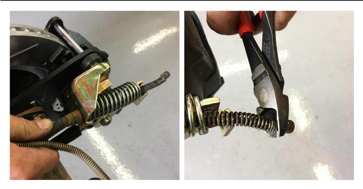
Depending on factory cable lengths, the existing cables can sometimes be used without any modification. If they are too long, then cut off the cable stop as shown using cable cutters or a cut-off wheel. The spring can be removed with the cable installed into the parking brake caliper as shown.
