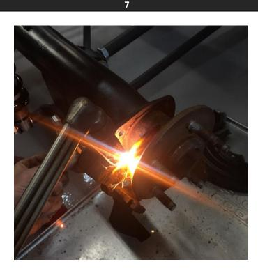
Remove the original caliper mounting bracket. Again, this can be done using any method you prefer.
