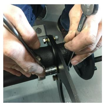
Bolt on the brackets using the supplied hardware as shown and torque to **20 ft-lbs**. Your caliper should be mounted to the **REAR** (back) of the axle. The brake hose bracket will be positioned with the tab to the front of the axle. All brackets are mounted on the inboard side of the axle flange.
