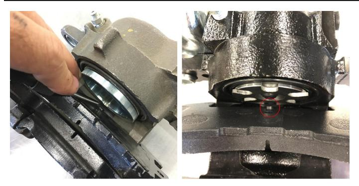
**Kits with non-parking brake calipers** should be checked to confirm the machined pad spacers are present and make sure the notch in the pad spacer lines up with the corresponding boss on the brake pad. **Kits with parking brake calipers** do not use a machined pad spacer and should be checked to confirm the pad is seated flat against the piston face, with the boss of the brake pad lining up with the notch in the piston face.
