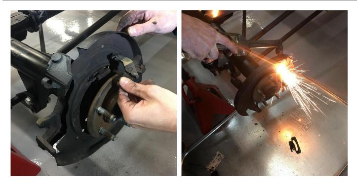
Disconnect and remove the parking brake cable and lever. The brackets in this kit are designed to be installed without removing the differential cover. This can be done by use of a cut-off wheel, reciprocating saw, or torch to split the backing plate into two pieces for removal. If you wish to retain your backing plates, the axles can be removed from the housing by draining the fluid, then removing the differential cover and the axle shafts.
