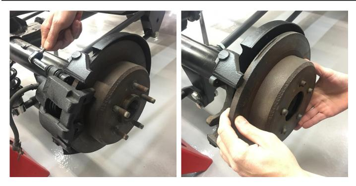
This installation refers to the **passenger side** of the axle (unless noted). All steps are to be repeated on the driver side. Start by removing the factory caliper and disc. It may be necessary use a lubricant around the axle register to do this, if corrosion is present.
